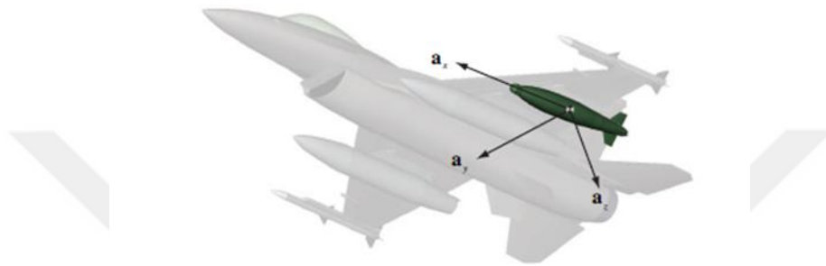
Figure 2.1 : Definition of aircraft axis coordinate system
