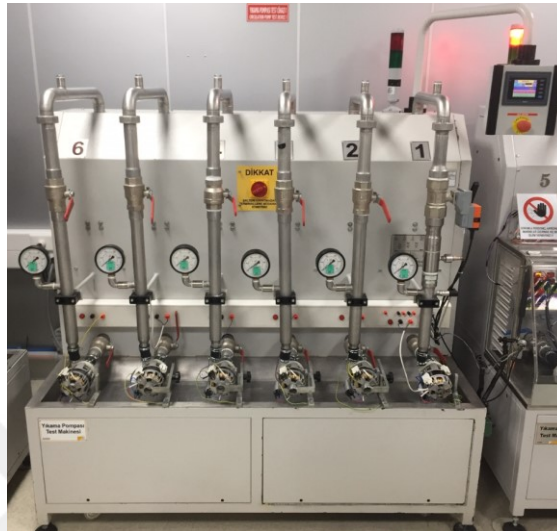
Figure 5.1. The Test Bench of the Evaluation of Performance of Pump
