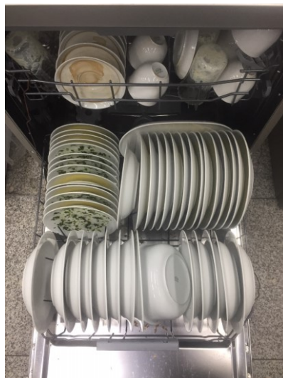
Figure 5.20. Loading Schematic and Soil for Cleaning Test
