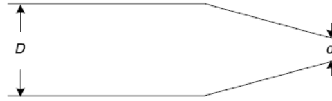
Figure 3.9. A Confusor Outlet (Source: Swamee, P. K., and Sharma, A. K., 2008)
