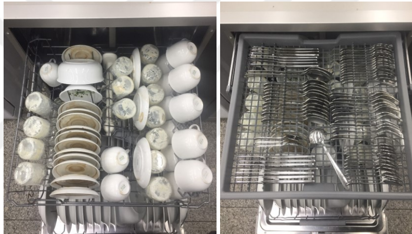
Figure 5.19. Loading Schematic and Soil for Cleaning Test
