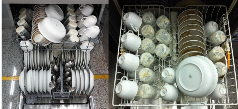
Figure 5.11. Loading Schematic of Vestel (Left) and Reference (Right) Dishwasher (Source: Internal Image)
