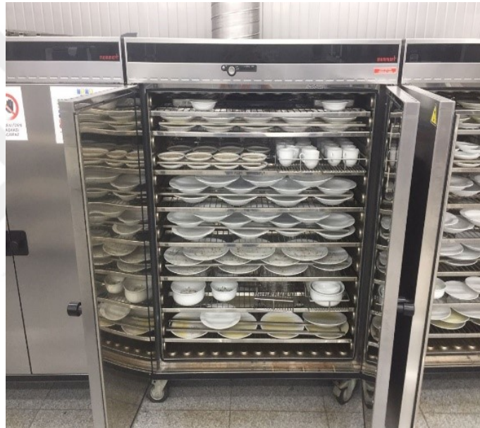
Figure 5.10. Preparation of Soil for Heating in the Furnace (Source: Internal Image)
