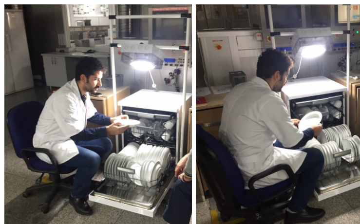
Figure 5.12. The Evaluation of the Cleaning and Drying Tests of the Dishwasher (Source: Internal Image)
