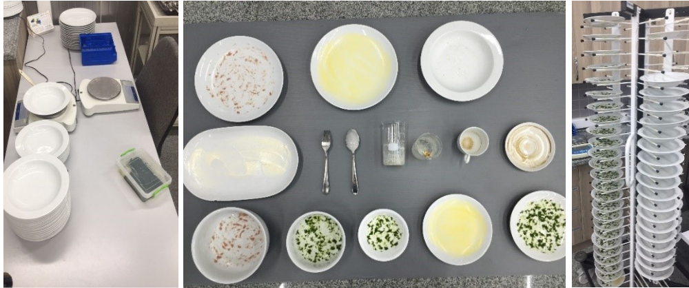
Figure 5.9. Preparation of Soil for Performance Test of Dishwasher (Source: Internal Image)
