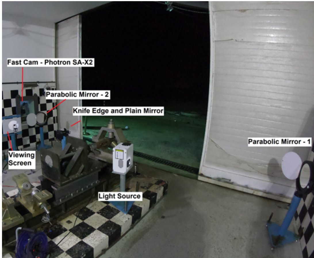
Figure 2.33: Schlieren layout on MAMTS
