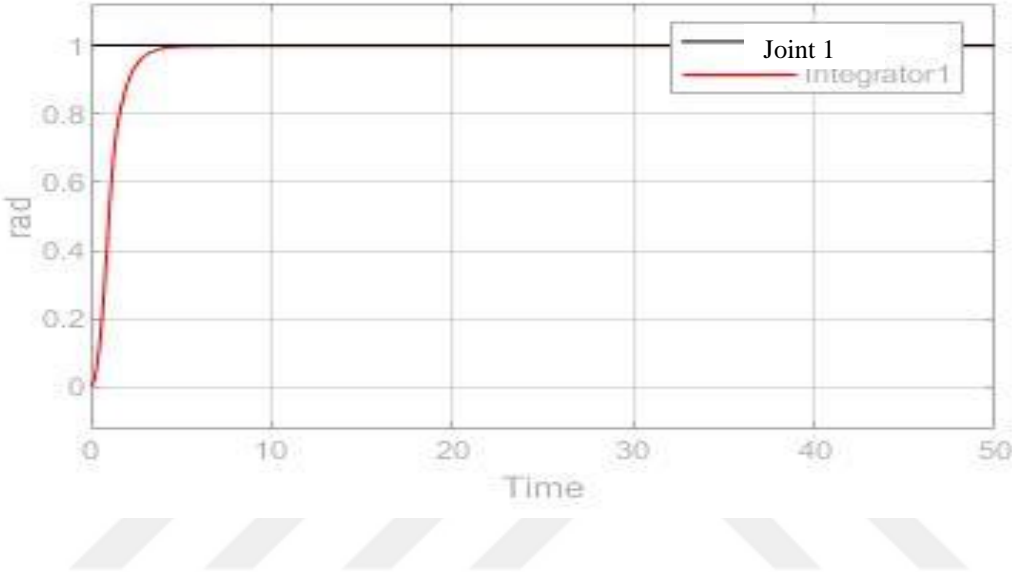
Figure 4.45: Joint 1 “critically damped” response of PD-CTC to step input.
