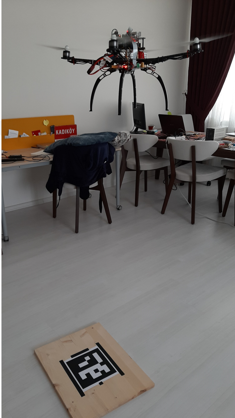
Figure 5.40: Photo of the quadrotor during path follow
