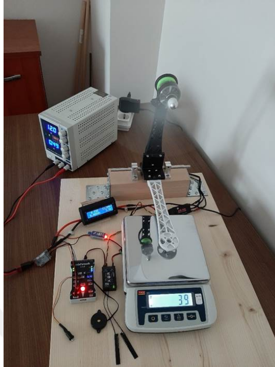
Figure 4.28: Thrust measurement setup for quadrotor motor-propeller pair
