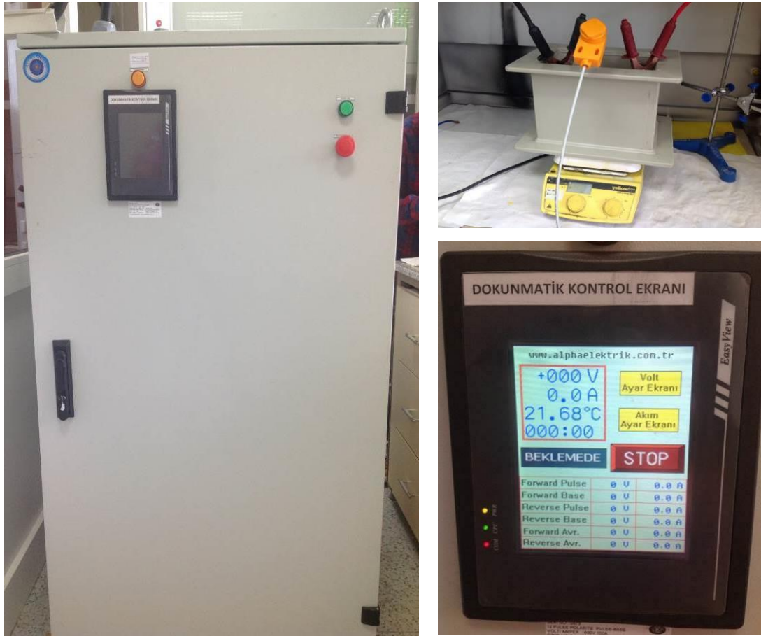
Figure 3.20 Redressor and final laboratory experimental setup in EMUM, DEU
