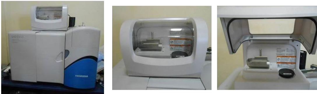
Figure 3.26 Horiba, LA-950 V2 type particle size analyzer in Mining Eng., DEU
