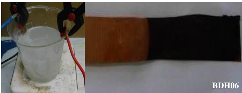
Figure 4.16 Cu cathode electrode of BDH06 after deposition
