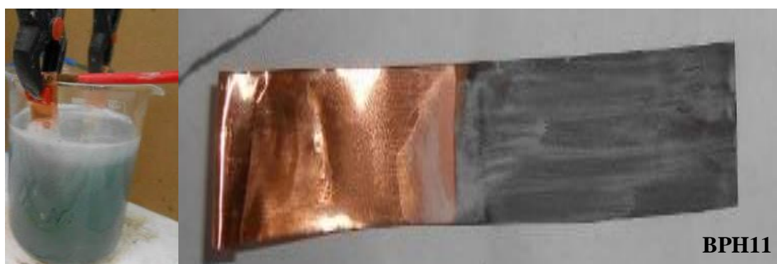
Figure 4.8 Cu cathode electrode of BPH11 after deposition
