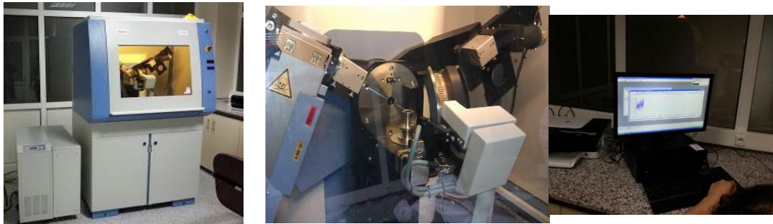
Figure 3.22 Thermo Scientific, Cu-K \alpha type XRD device in EMUM, DEU
