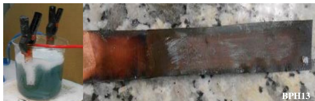
Figure 4.9 Cu cathode electrode of BPH13 after deposition
