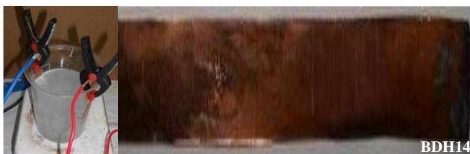
Figure 4.19 Cu cathode electrode of BDH14 after deposition
