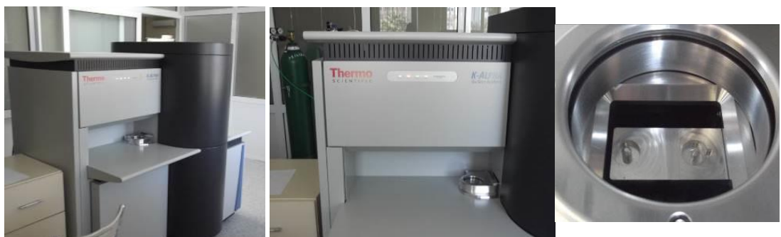
Figure 3.23 Thermo Scientific, K \alpha Surface Analysis type XPS device in EMUM, DEU
