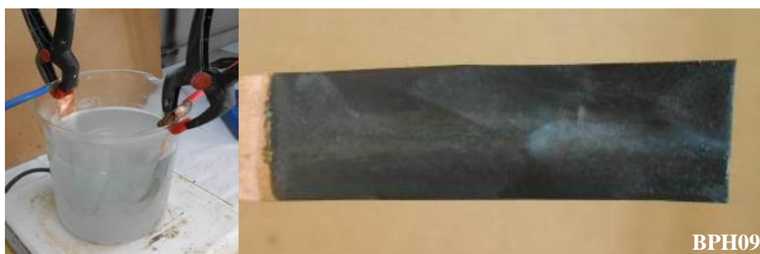
Figure 4.6 Cu cathode electrode of BPH09 after deposition
