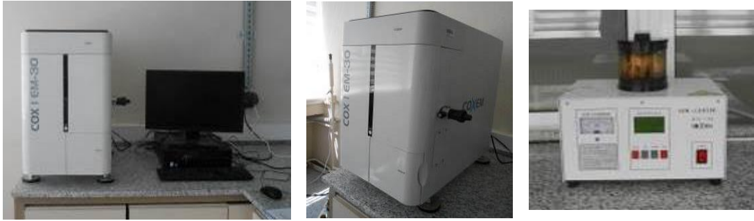
Figure 3.24 Coxem, EM-30 SEM with ion coater in EMUM, DEU
