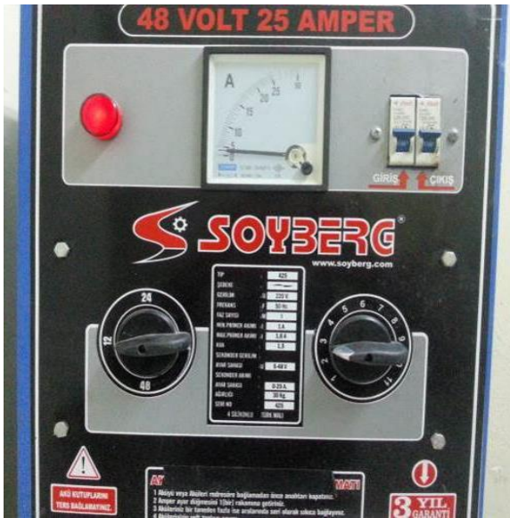
Figure 3.17 Redressor and preliminary experimental setup in IMYO, DEU
