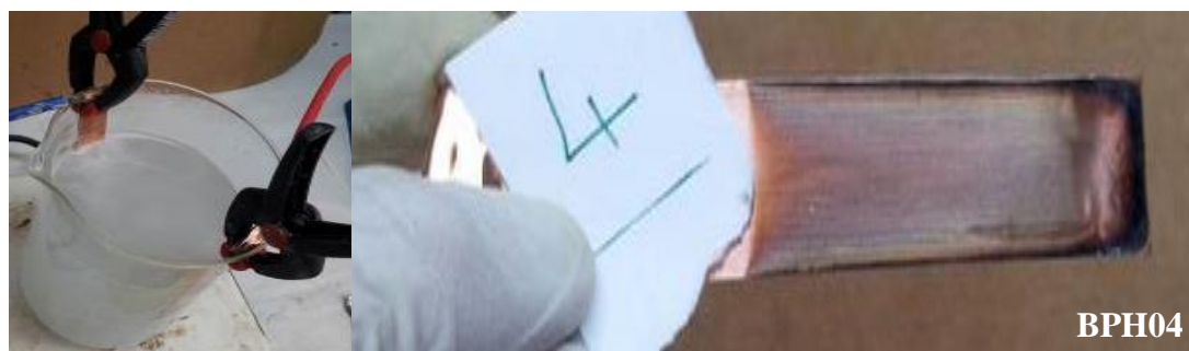
Figure 4.5 Cu cathode electrode of BPH04 after deposition
