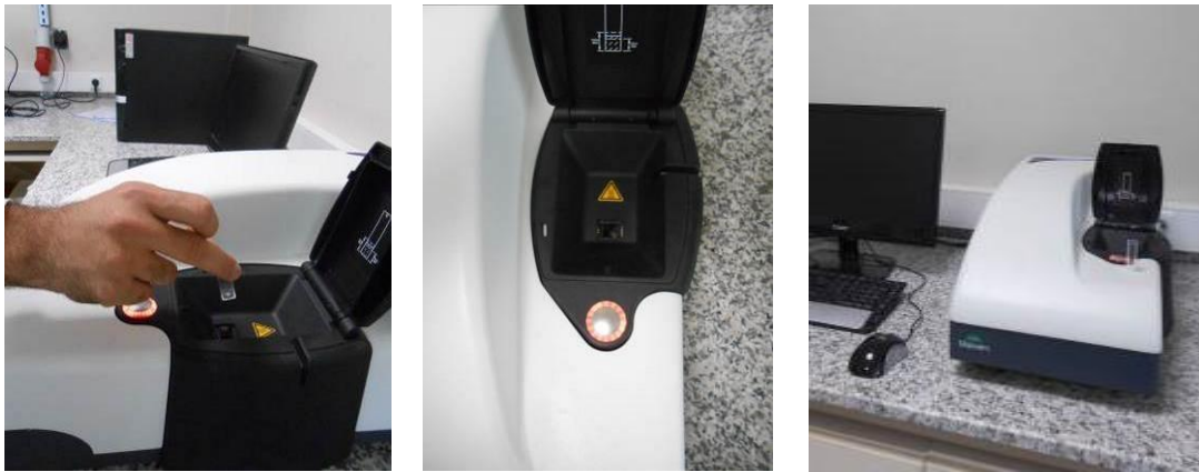
Figure 3.25 Malvern, Zetasizer Nano Z type nano particle size analyzer in EMUM, DEU
