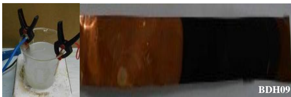
Figure 4.17 Cu cathode electrode of BDH09 after deposition
