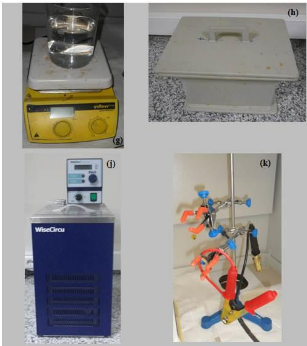
Figure 3.21 Auxiliary laboratory equipment in electro-deposition experimental setup (a) high-energy ball mill, (b) agate mortar, (c) pH meter, (d) analytical balance, (e) water purifier, (f) mechanical stirrer, (g) magnetic stirrer and heater, (h) polypropylene bath, (j) water circulator, (k) wire stand and clamps
