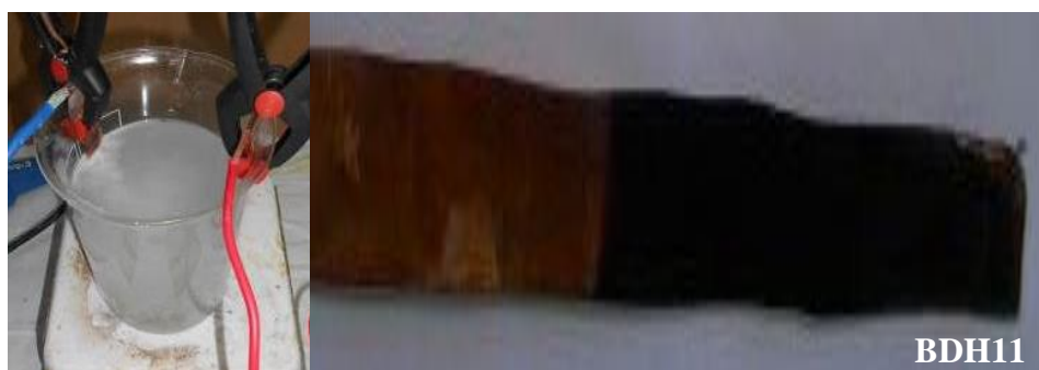
Figure 4.18 Cu cathode electrode of BDH11 after deposition
