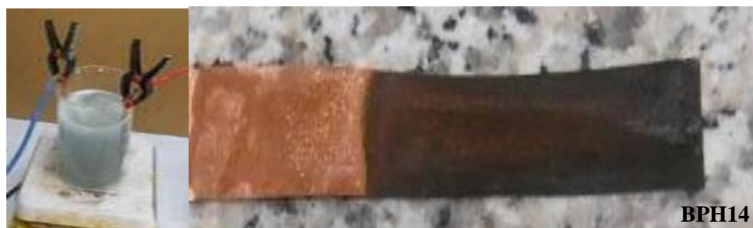
Figure 4.10 Cu cathode electrode of BPH14 after deposition
