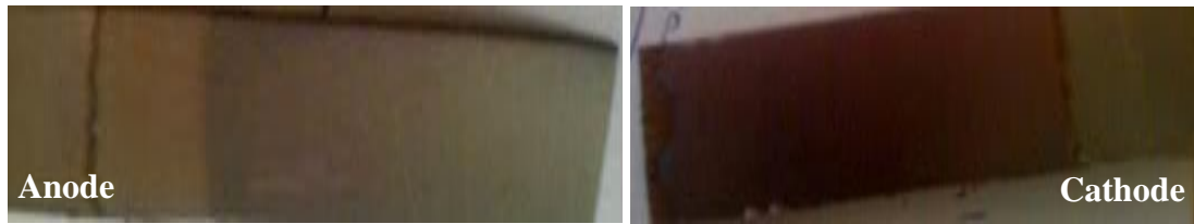
Figure 4.13 Ti anode and cathode electrodes of BPH31 after deposition
