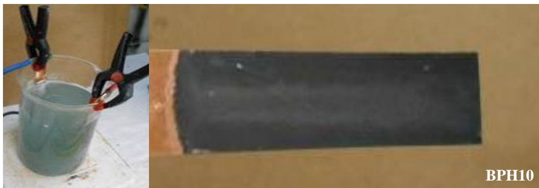
Figure 4.7 Cu cathode electrode of BPH10 after deposition
