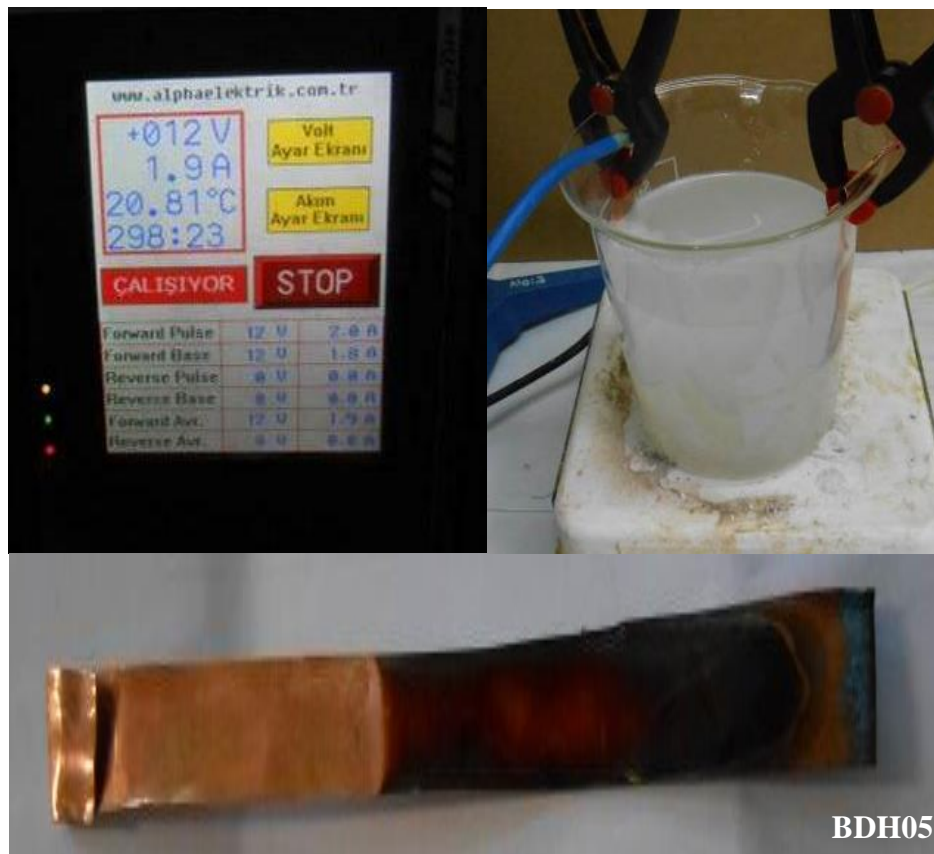
Figure 4.15 Cu cathode electrode of BDH05 after deposition
