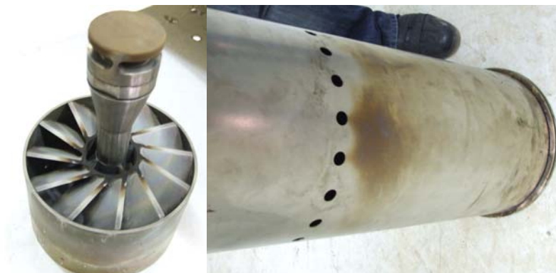
Figure 6.9 Injector with Swirler and Liner After the 3 rd Test
