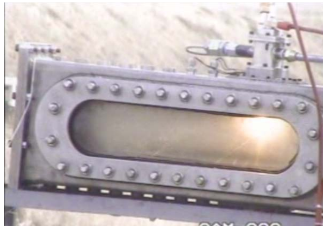
Figure 6.4 Firing of the Pilot Flame Igniter During the Characterization Tests
