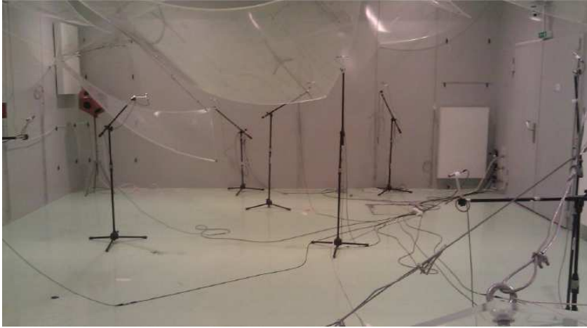
Figure 2.9 Reverberation room reflectors, microphones and sound source (Kırbaş, 2013).
