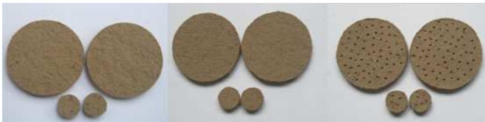
Figure 2.27 A set of specimens with various finishing; rough surface (left), screen surface (middle) and perforated surface (right) (Sihabut & Laemsak, 2012)
