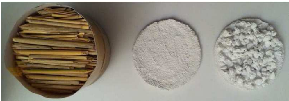
Figure 3.3 Layers of the configuration: left: reed (R1), center: small diameter pumice aggregate (F1) and right: wider pumice aggregate (B1).
