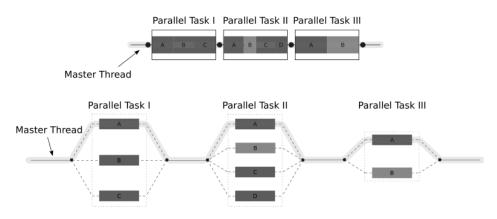
Figure 3.1 : An illustration of Multithreading.
