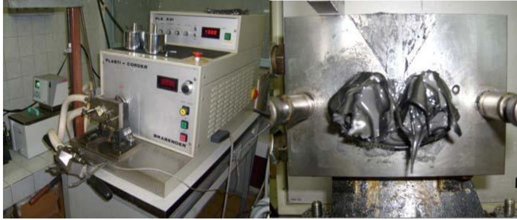
Figure 3.1 General view Brabender Plasticorder W30/The mixing chamber and the rotors after the mixing process of the composite (Çolak, 2011).
