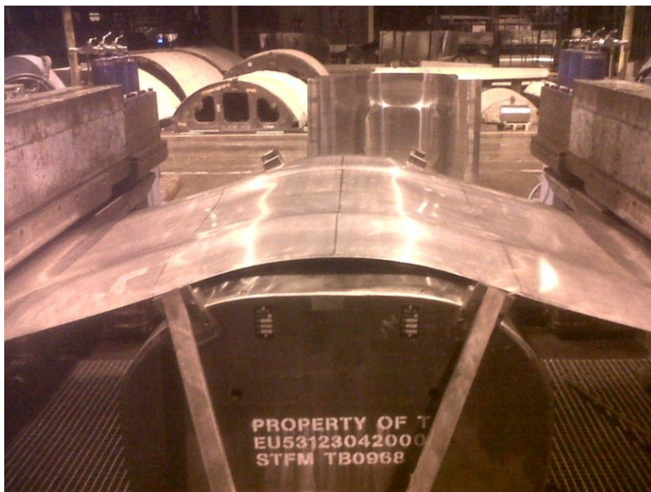
Figure 98: Experimental trial to form cockpit part in 750 tons capacity Cyril-Bath press
