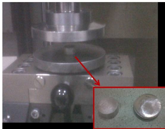
Figure 42: Stack compression test set-up and test specimen
