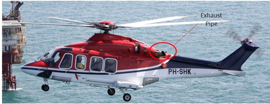
Figure 102: Exhaust pipe location in AGUSTA AW-139 Helicopter
