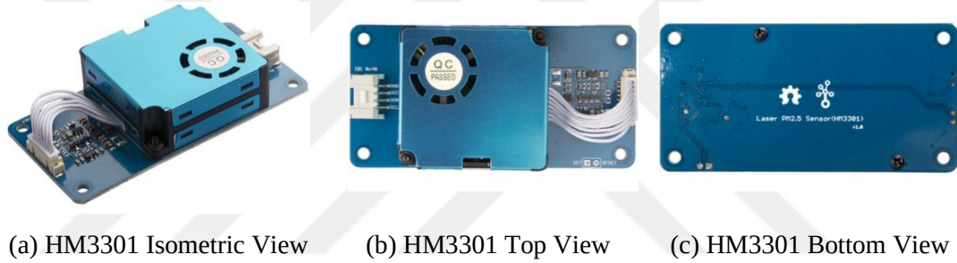
Figure 3.2 The Isometric (a), Top (b), and Bottom (c) Views of the PM_{2.5} Sensor - HM3301
