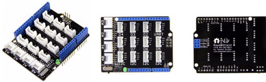
(a) Grove Base Shield V2.0 Isometric View (b) Grove Base Shield V2.0 Top View (c) Grove Base Shield V2.0 Bottom View
