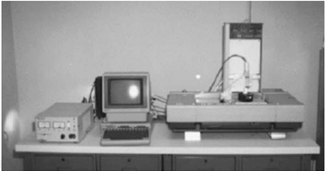
Figure 2.12 The First AM Technology from Hull (Gibson et al., 2015, p.38)
