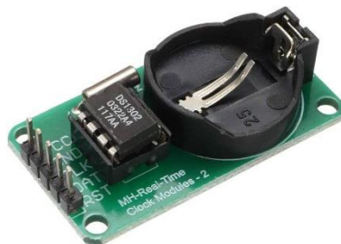
Figure 3.22 The Visual of the Real-Time Clock - DS1302
