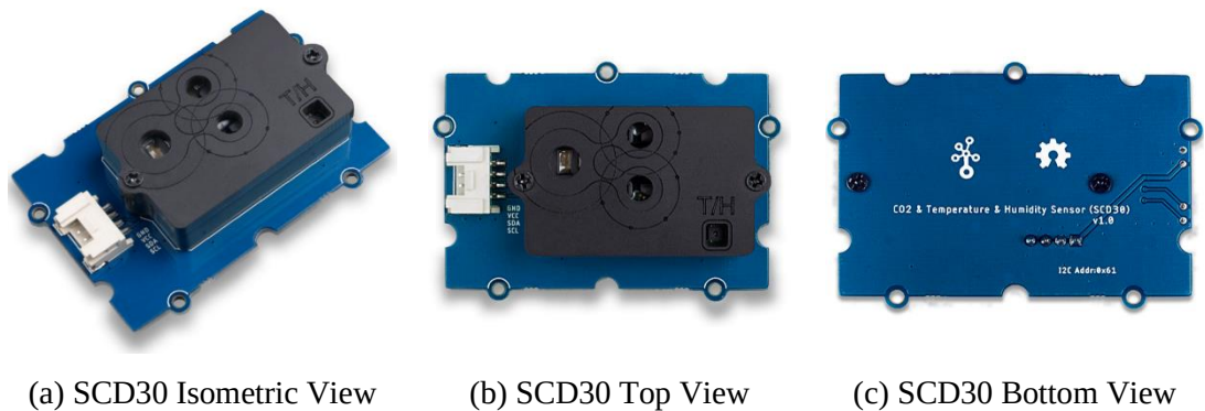
Figure 3.7 The Isometric (a), Top (b), and Bottom (c) Views of the CO 2 Sensor - SCD30
