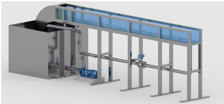
Figure 2.2. Schematic view of the open channel system
