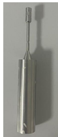
Figure 2.5. Viscometer used for viscosity determination.
