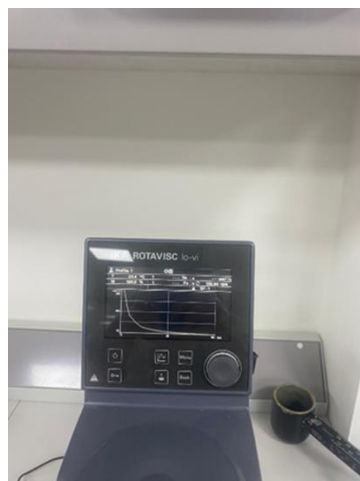
Figure 2.5. Viscometer used for viscosity determination.
