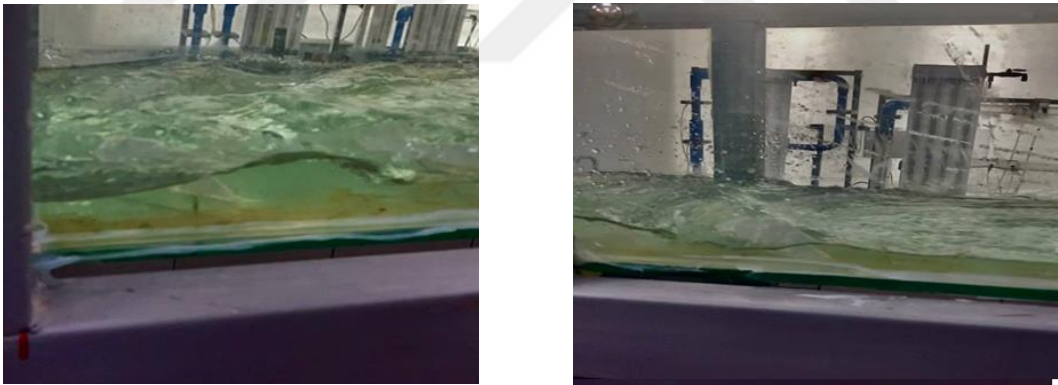
Figure 3.56. Depth profile in first obstacle explaining the flood jump, a) S = 1.0156^\circ , \dot{Q} = 0.0035 \text{ m}^3/\text{s}
