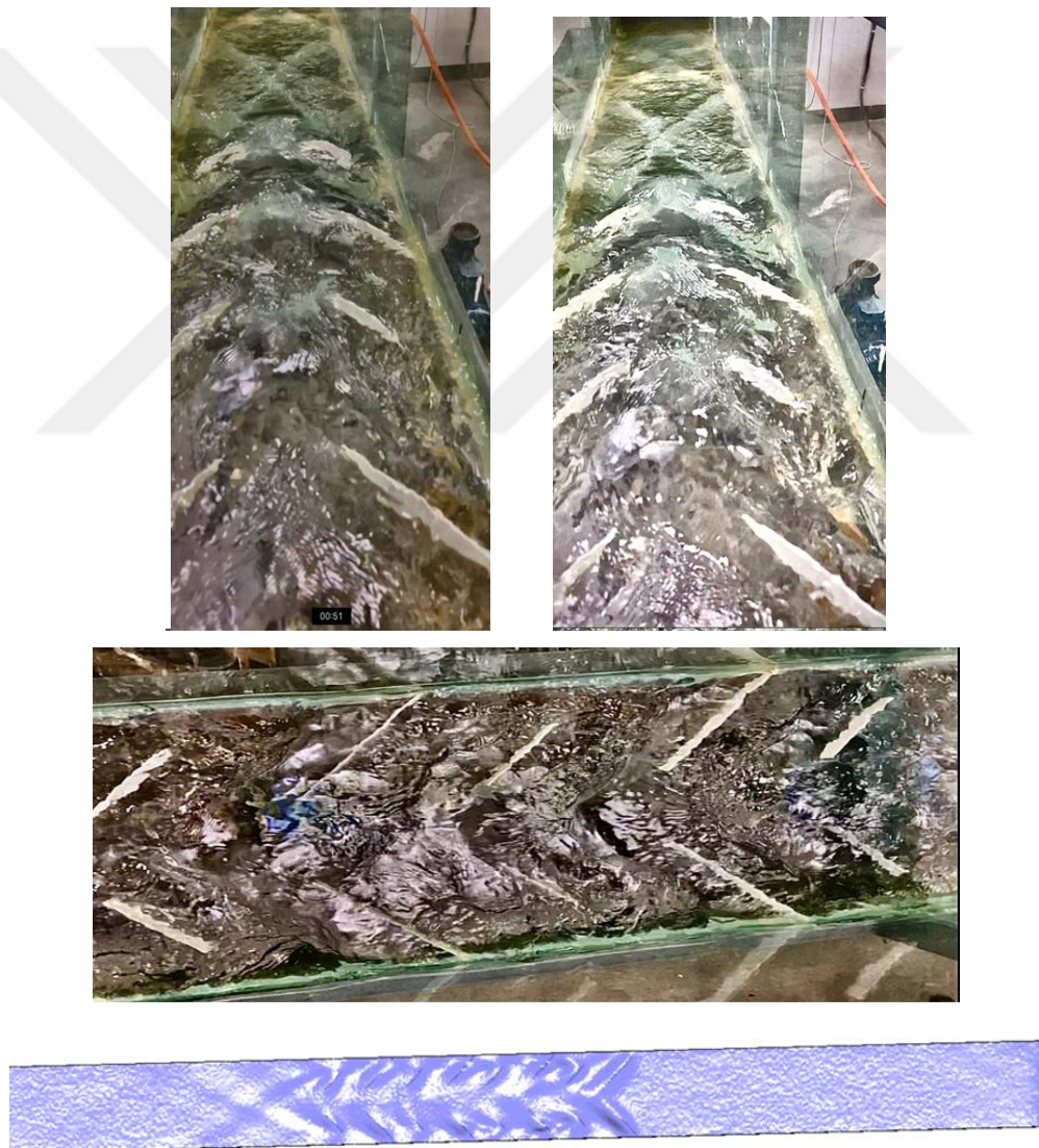
Figure 3.54. Water profiles from top view S = 1.406^\circ , \dot{Q} = 0.0045 \text{ m}^3/\text{s}
