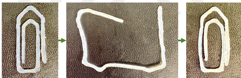
Figure 4.12 : 4D-printed paperclip-shaped hydrogel with 50 mol% C16A and 0.5 x_{DMAA} . From left to right: as prepared state, programmed temporary shape, and recovered permanent shape.
