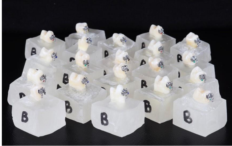
Figure 6: Group B - 20 specimens with TiO 2 nanoparticles incorporated in the composite adhesive
