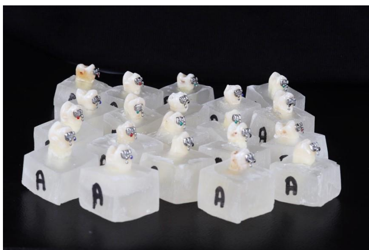
Figure 5: Group A - 20 specimens with TiO 2 nanoparticles incorporated in the bonding agent
