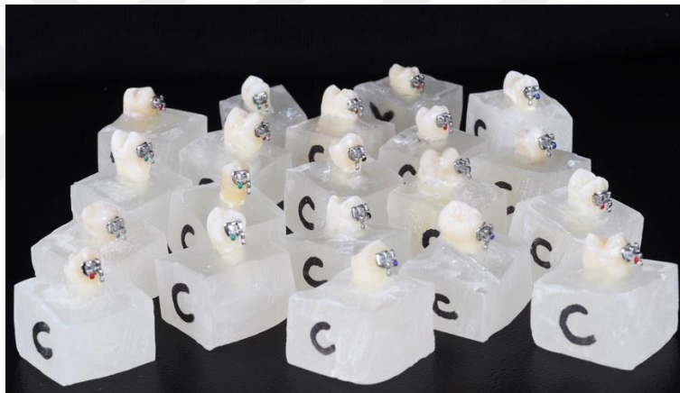
Figure 7: Group C - 20 specimens with conventional bonding agent and composite adhesive (no nanoparticles).
