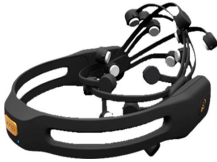
Figure 4. Saline solution EEG device (Crawford, Andujar, Remy& Gilbert, 2014).
