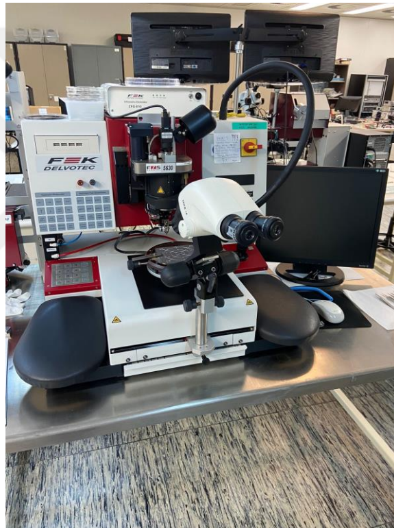
Figure 3.5. F&K Delvotec Wedge 5630 wire bonding system.
