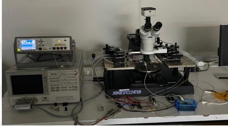
Figure 3.10. C-V measurement setup.
