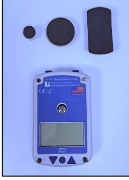
Resim 3.2. Lafayette® Model-01165 hand-held dinamometre
