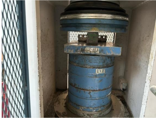
Figure 4.15 Compressive Strength Test.
