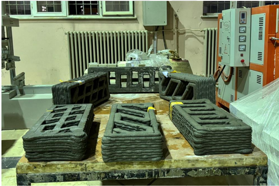
Figure 5.1 Hollow concrete beams of M1 and M2 before measuring their heights.
