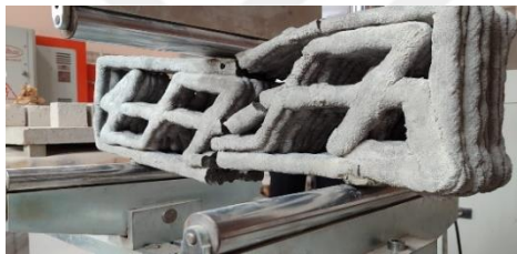
Figure 5.2 Different internal pattern and different crack propagation path.
