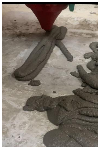
Figure 4.6 Very high workability causes problems.
