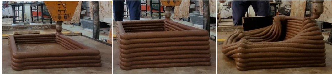
Figure 2.14 A square section element printed by Imran et al. [24].
