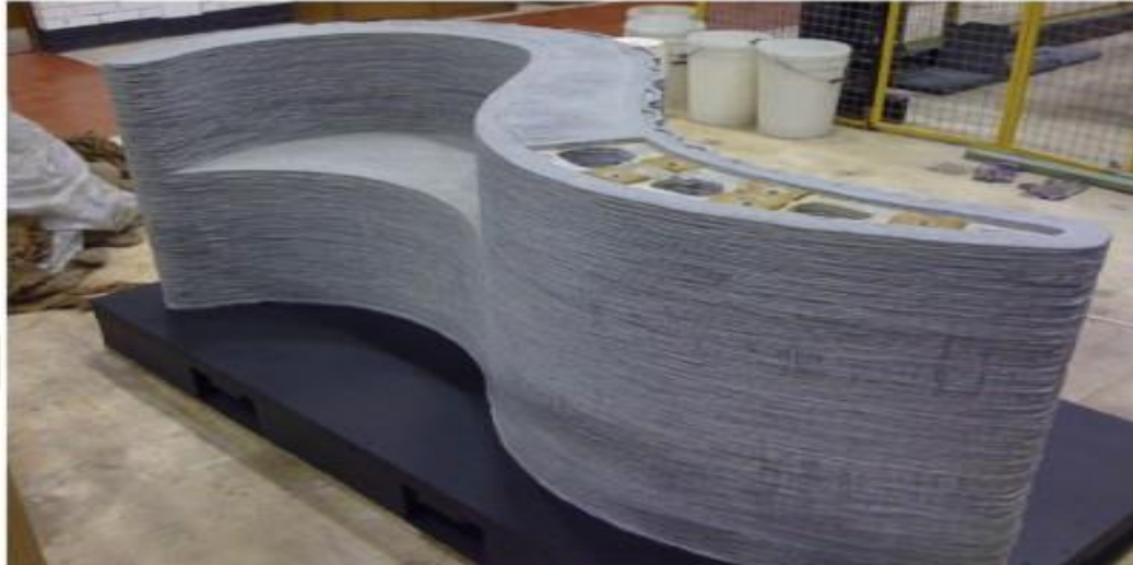
Figure 2.2 Concrete Printing method.
