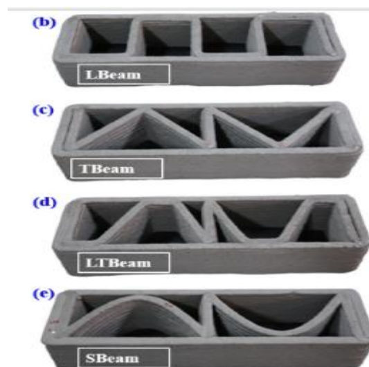
Figure 2.13 Structural elements with internal patterns printed by Dey et al. [23].
