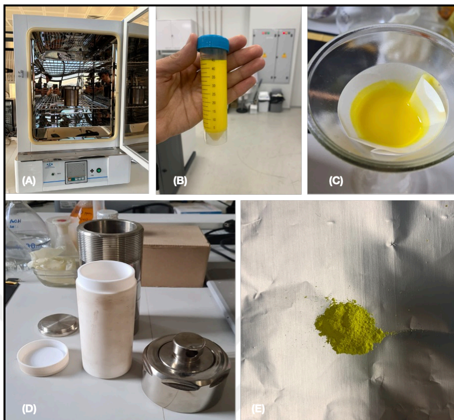
Figure 3.2 Images of (A) teflon-coated stainless-steel autoclave to be kept in the oven at 180°C for 24 hours, (B) solution obtained after autoclave, (C) filtration of the solution, (D) autoclave system used in the synthesis, and (E) obtained Cd_xZn_{1-x}S catalyst.
