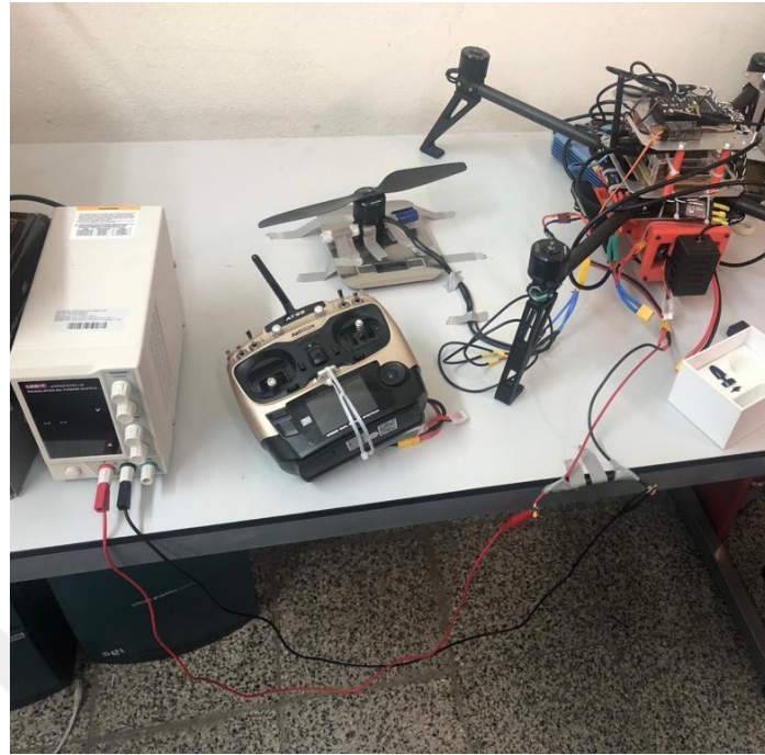
Figure 8.2. Experimental setup for measuring current correlation with different lift values.
