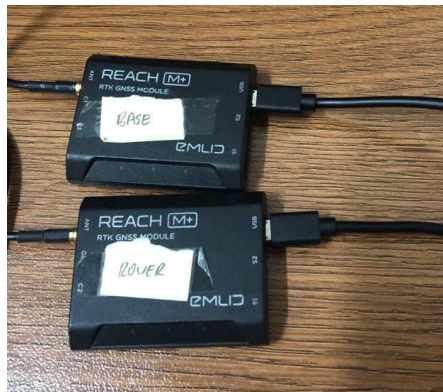
Figure 3.7. Reach M+ RTK-GNSS module.
