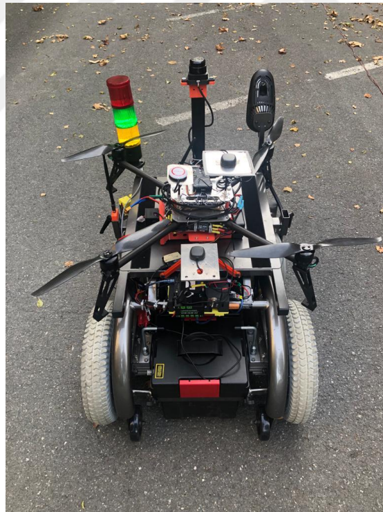
Figure 8.7. Drone mounted on the UGV.
