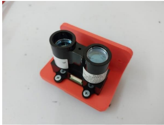
Figure 3.4. Garmin Lidar-Lite V3 optical distance sensor.
