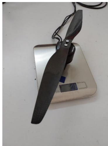
Figure 8.1. Experimental setup to measure lift generated by each rotor at full throttle.
