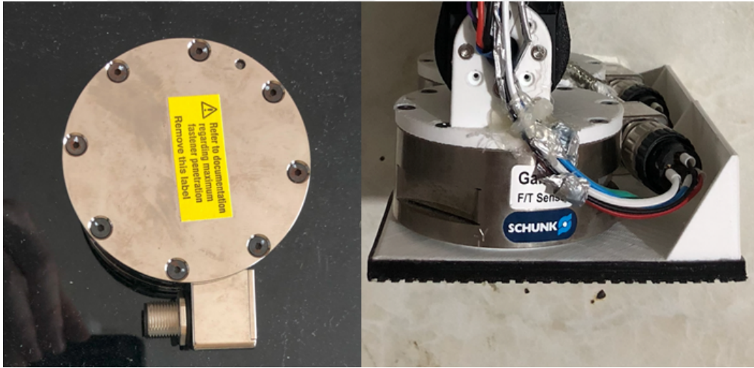
Figure 3.28: The sensor is shown from the top at left image, and the places of sensors at the robot feet is shown at the right.
