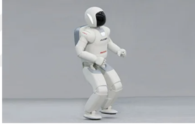
Figure 3.1: Robot ASIMO is shown in the picture, where knees are half-closed while it stands up because of the constraint introduced by its locomotion algorithms [56].
