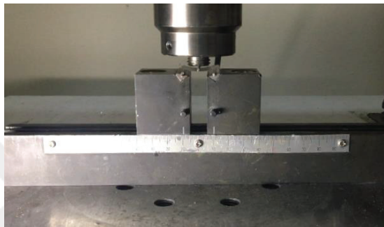
Figure 4.8. The test setup for three-point bending test
