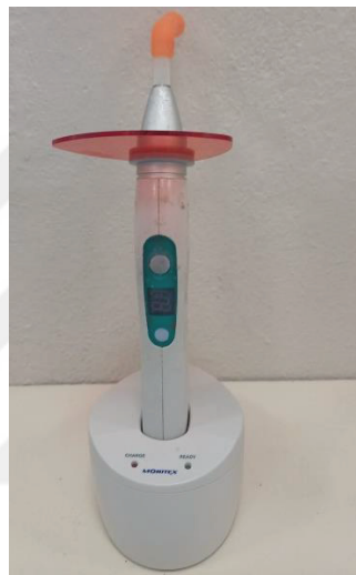
Figure 4.5. Light curing unit used in the curing process
