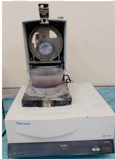
Figure 4.4. Automatic mortar mill for homogeneous dispersion of the particles
