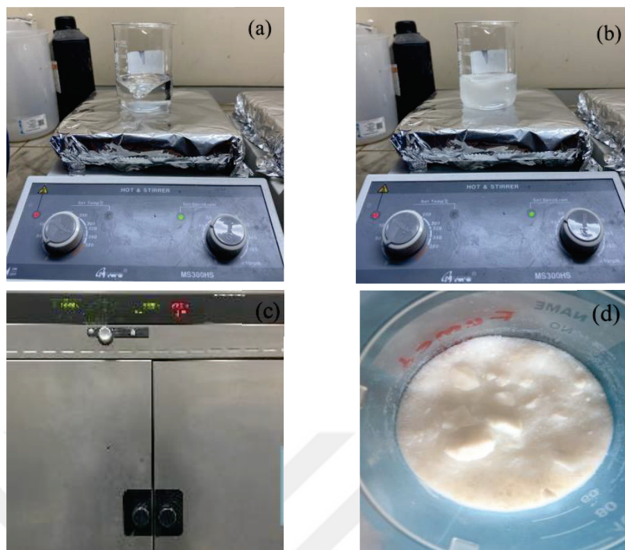
Figure 4.2. Surface modification process of the nanoparticles; (a) chemical mixture, (b) particle addition to chemical mixture, (c) remove the volatile chemicals at 80°C for 24 hours, (d) surface modified particles
