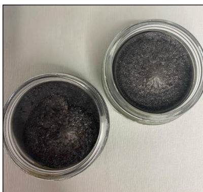
Figure 4.3: The structure of the lyophilized OMA-PPy polymer.
