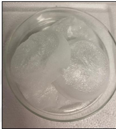
Figure 4.1: The structure of the lyophilized OSA polymer.
