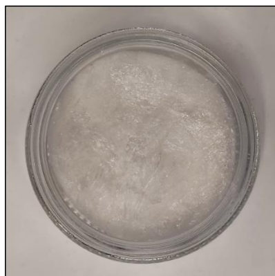
Figure 4.2: The structure of the lyophilized OMA polymer.
