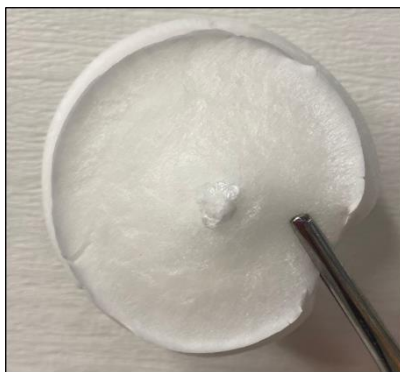
Figure 4.5: The structure of the lyophilized GelMA polymer.
