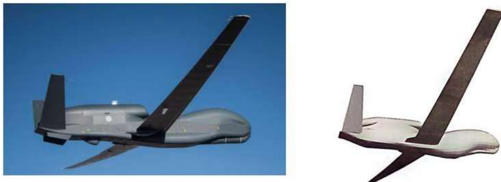
Figure 2.31 : The photo at the left: actual flight, at the right: ZONAIR solution.
