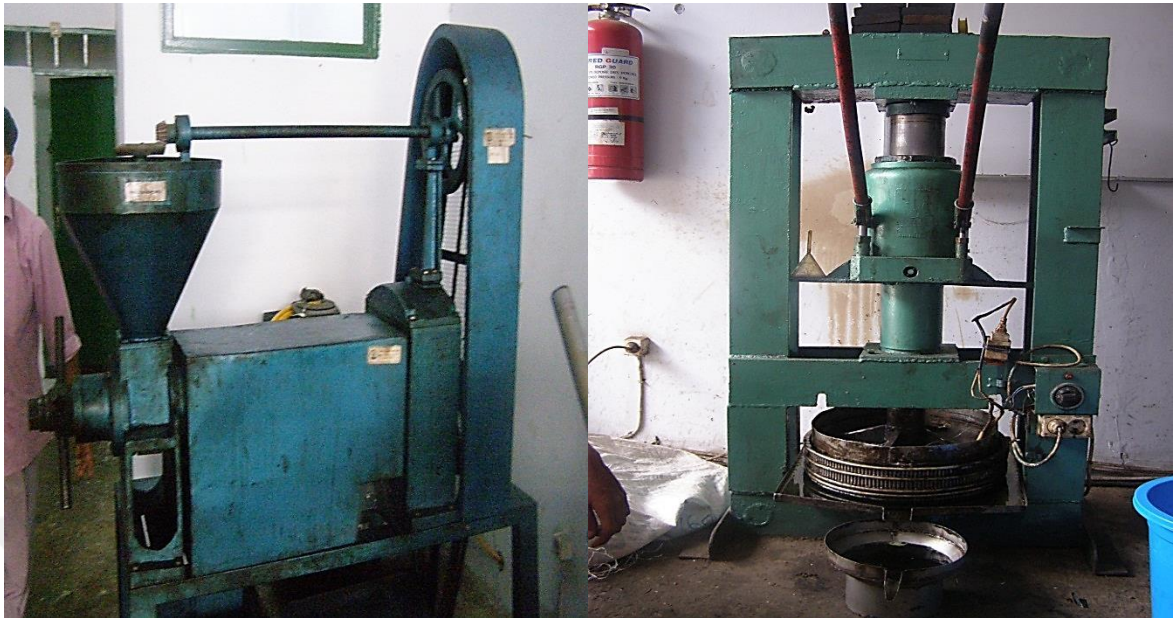
Figure 3.3: Screw extruder machine and hydraulic manual pressing machine
