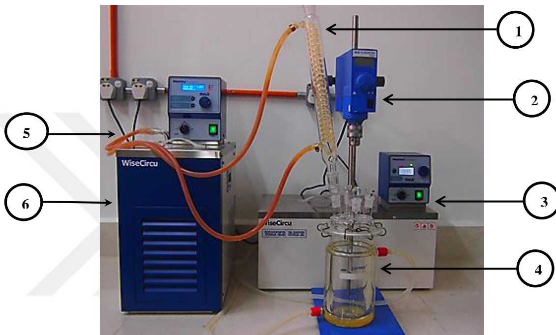
Figure 3.6: Experimental set up used to perform biodiesel production (1) reflux condenser; (2) overhead mechanical stirrer; (3) circulating water bath; (4) Jacketed glass batch tank reactor (1 l); (5) hoses; (6) Refrigerator
