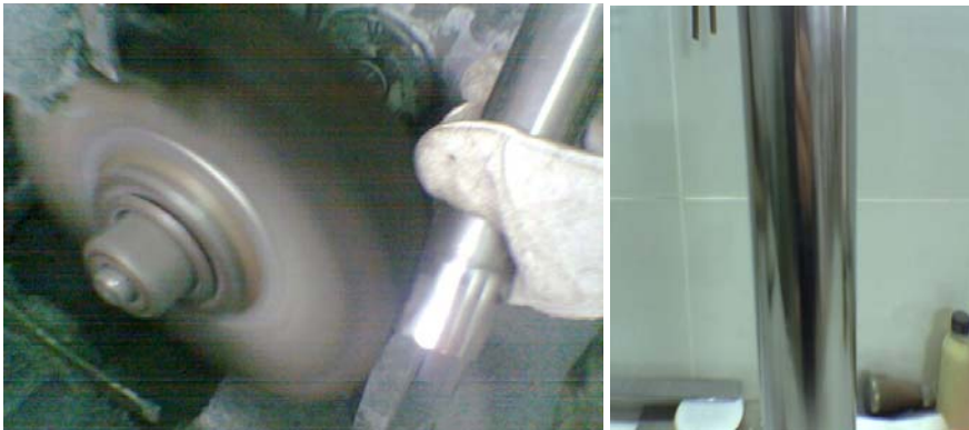
Figure 3.8. The pipe treated with boric acid was coated with chromium after polishing.
