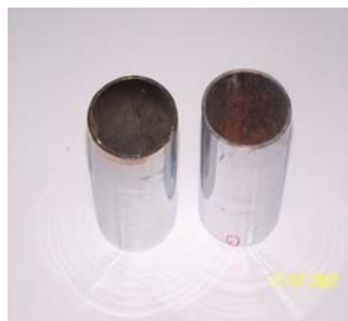
Figure 3.10. Corrosion resistance of pipe specimens after salt spray test.
