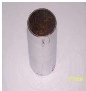
Figure 3.9. The pipe specimen cleaned with cyanide.
