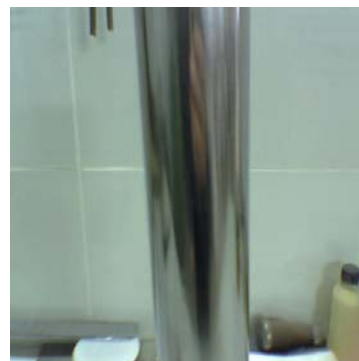
Figure 3.3. Chromium coated pipe specimen
