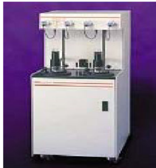
Figure 4.11: Mercury porosimetry equipment [48]
