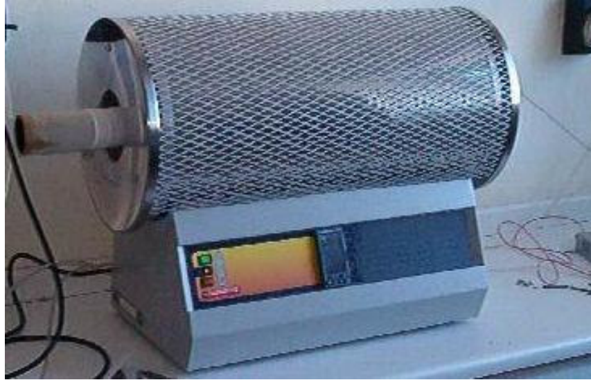
Figure 4.9: The temperature – programmed furnace where the stabilization and carbonization processes occur [48].
