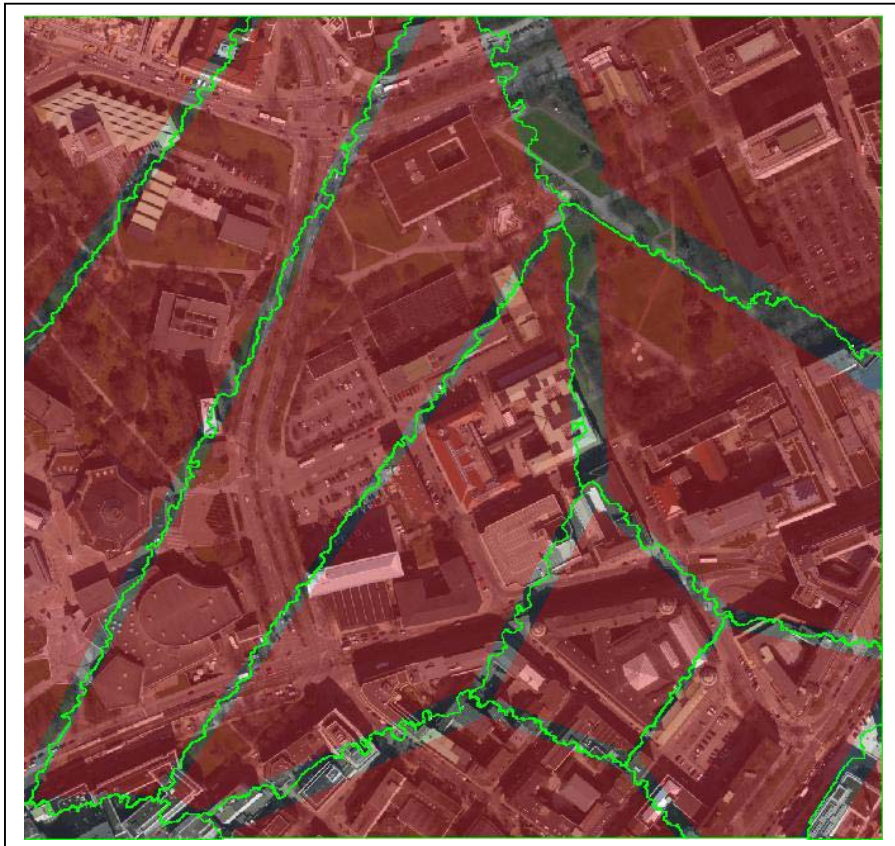
Figure 4.5: (b). Seamline definition for merging orthophotos
