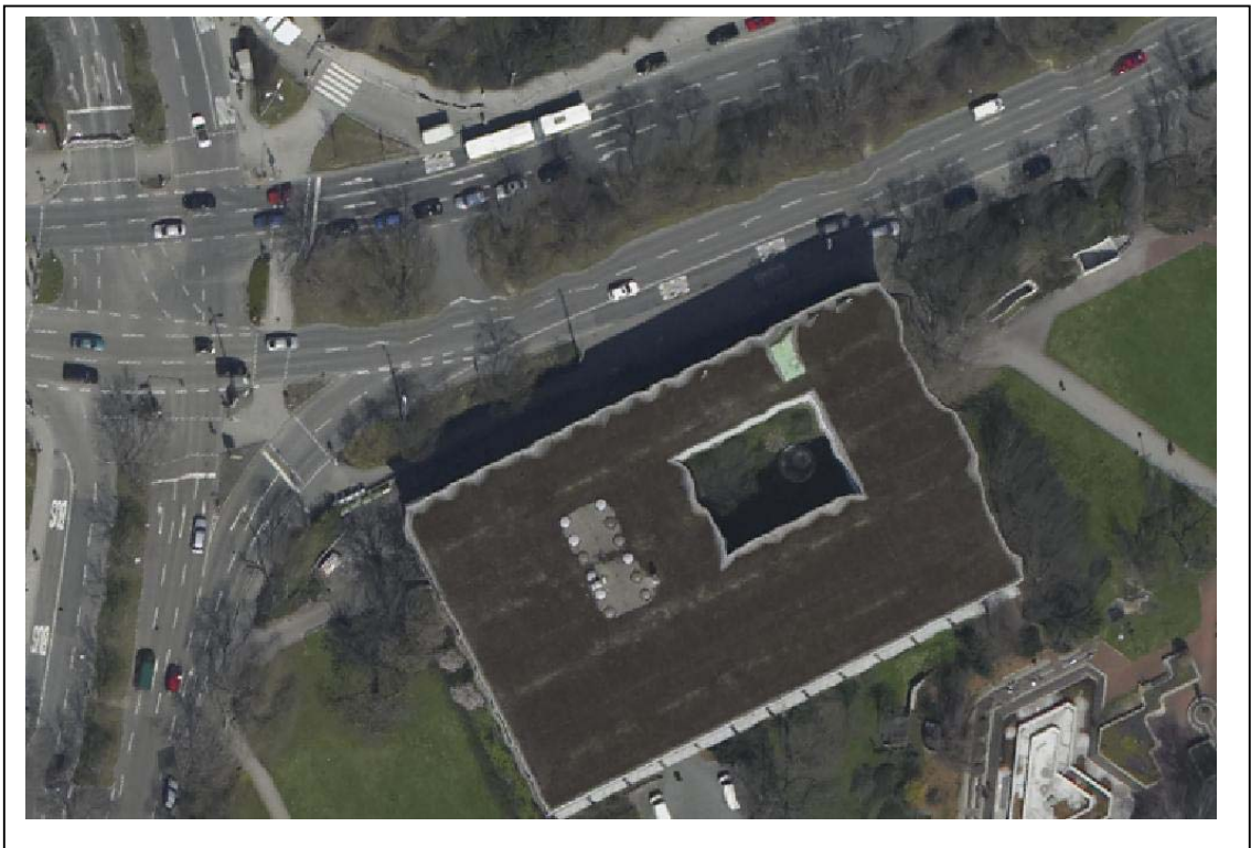
Figure 5.2: (a). True ortho photo from first pulse (0.25 cm pixel, 2m dense DSM)
