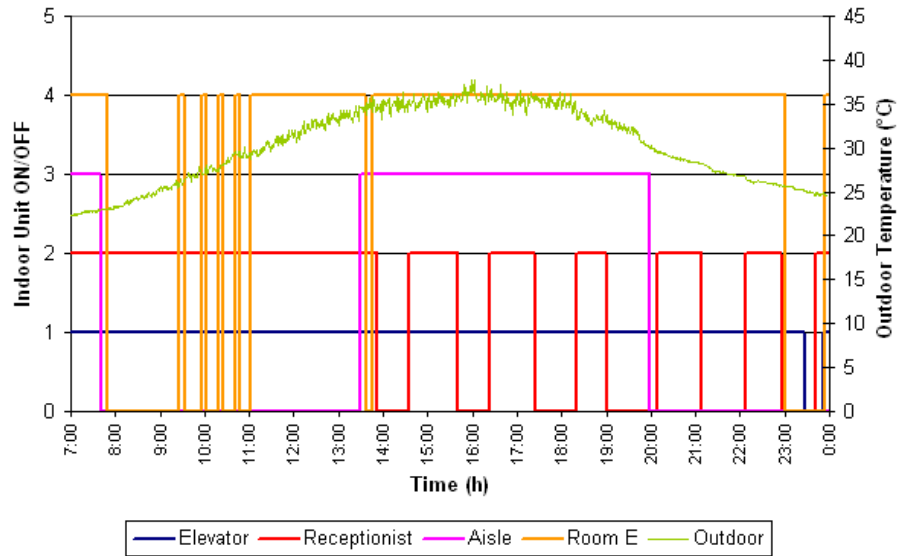
Figure 6.15 : Indoor units operation of System2 zones in individual control mode on June 01, 2007
