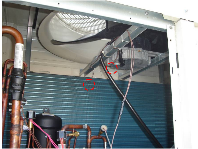
Figure 4.29 : Measurement location of the outdoor unit air outlet temperature
