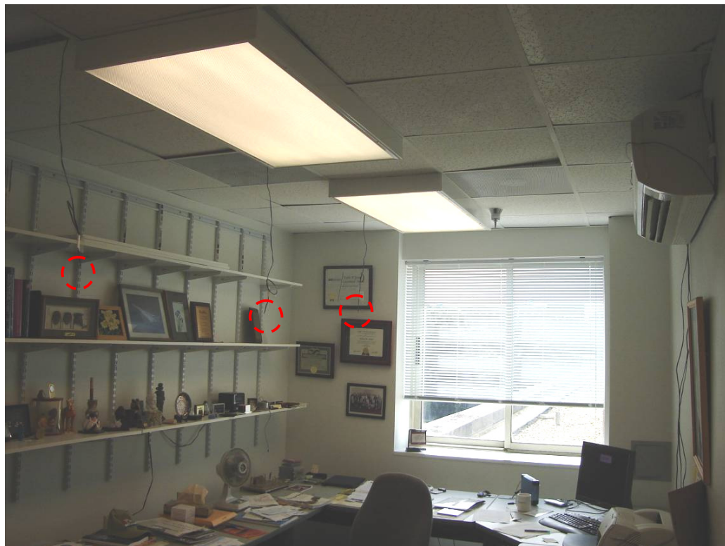
Figure 4.25 : Measurement locations: 1m away from the walls
