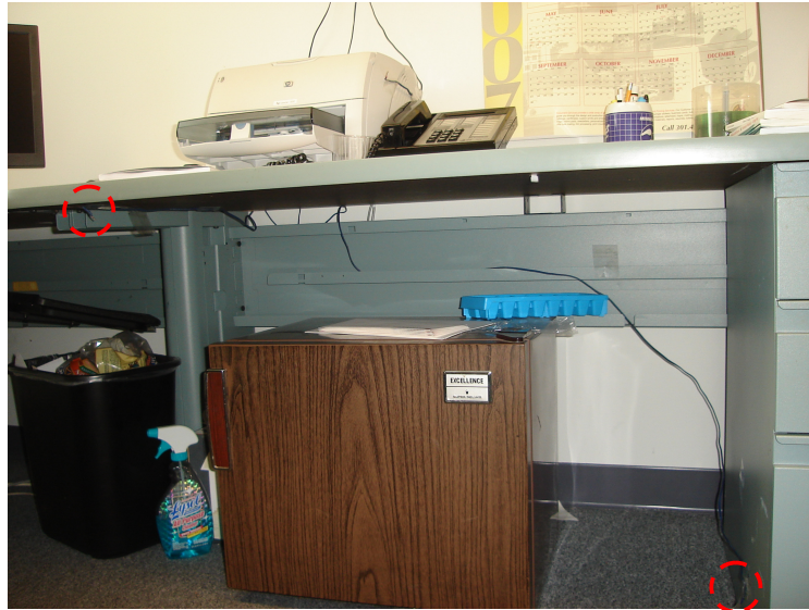
Figure 4.24 : Measurement locations of the occupant location: 0.1m and 0.6m above the floor
