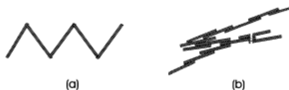
Figure 7. Alternative models describing the association of clay particles a) edge-to-edge (EE) ribbons; and b) 'Bandermodel' [22].
