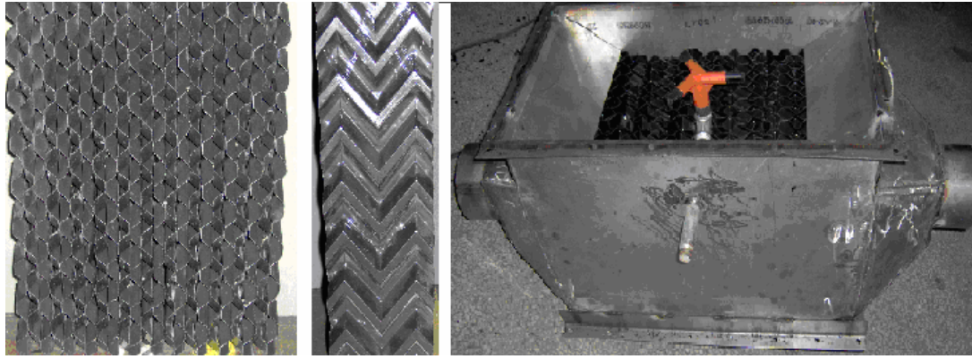
Figure 4.5 Different views of the pad humidifier.
