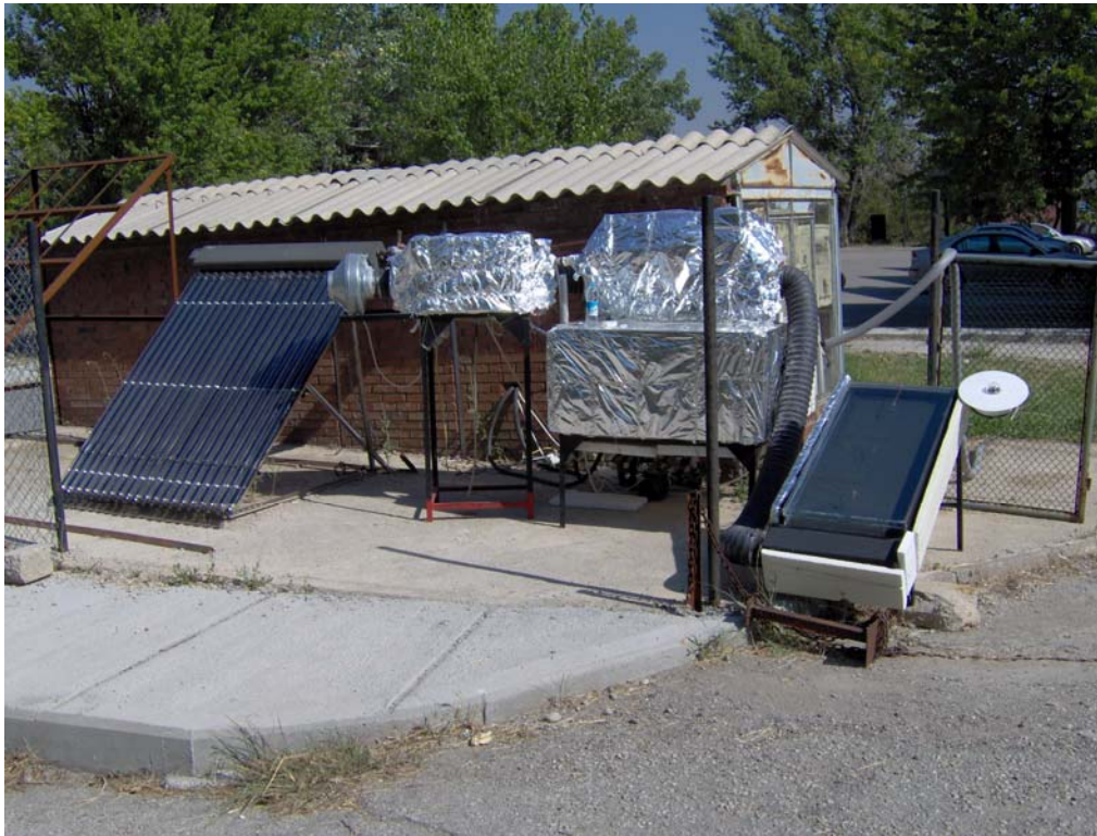
Figure E.1 A view of the desalination system integrated with an evacuated tubular water heater unit.
