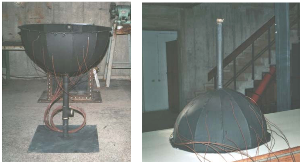
Figure 4.2 Bottom and Top Pieces of The Absorber
