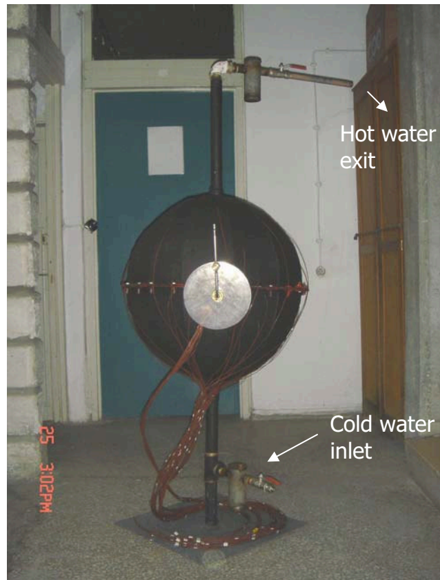
Figure 4.1 A General View of The Collector without Glass Covers
