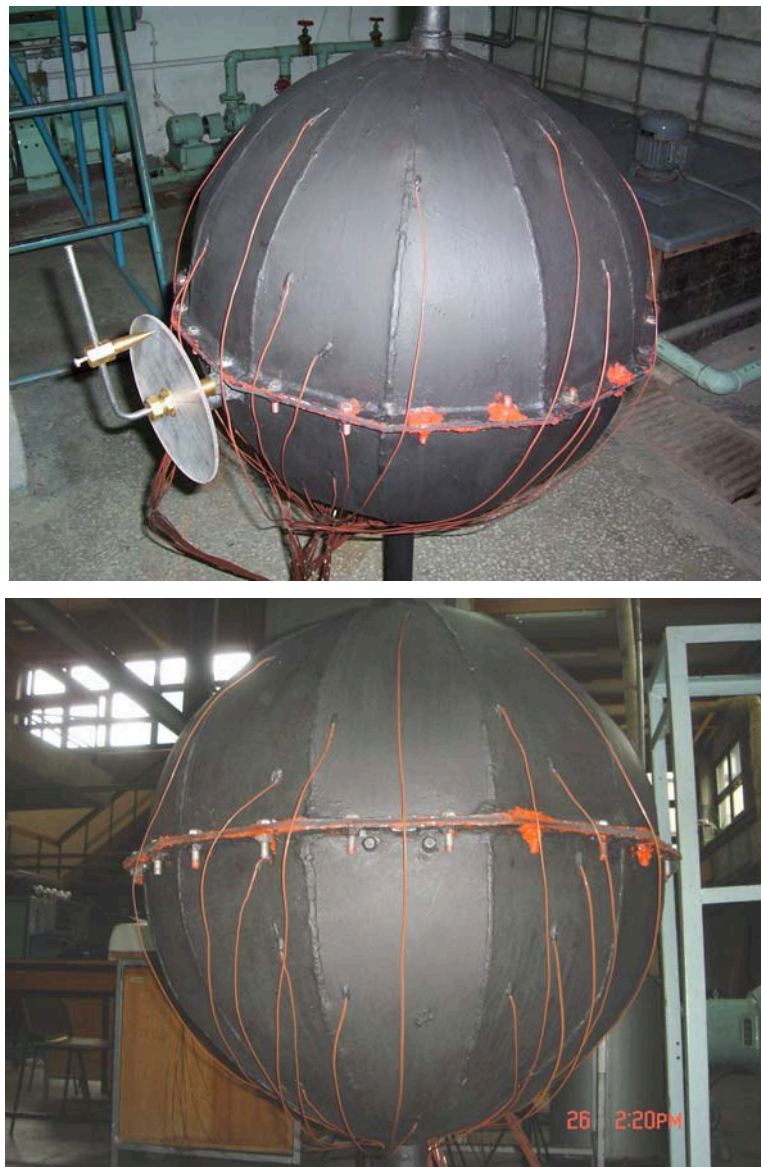
Figure 5.6 Thermocouple Locations on the Absorber
