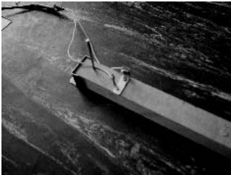
Figure 5.3 Device designed to detect start/end of scan (enable circuit).
