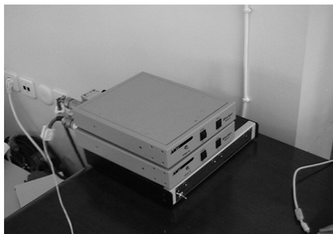
Figure 2.7 Motion Lab Systems EMG Amplifier and data acquisition system [2].
