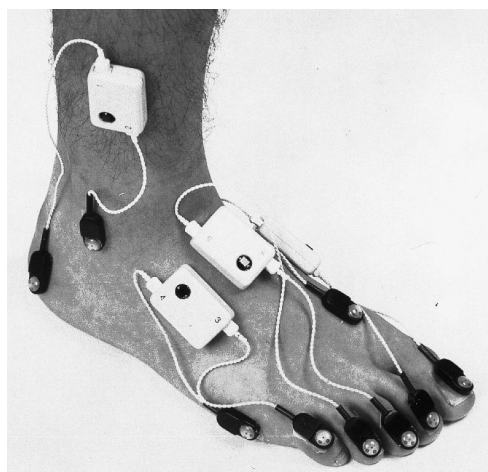
Figure 2.2 Light-emitting diode (LED) motion markers [1].
