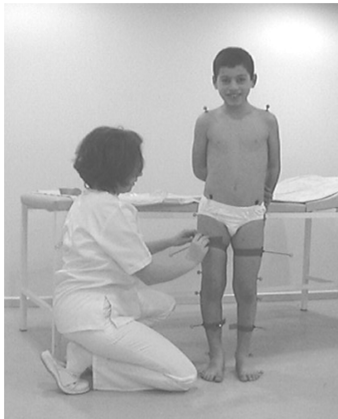
Figure 3.1 Davis model based marker setup in Motion Analysis Laboratory [4].
