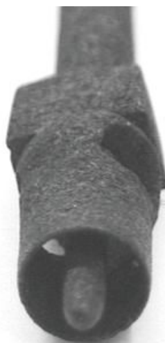
Figure 23 Graphite anode with its extension rod.
