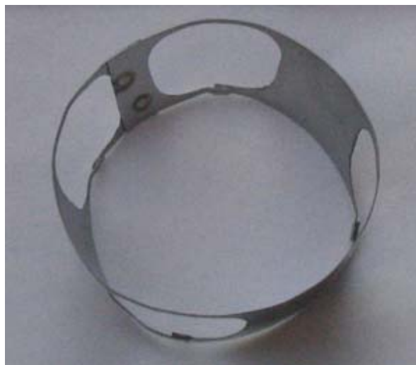
Figure 24 Stainless steel cathode without extension rod.
