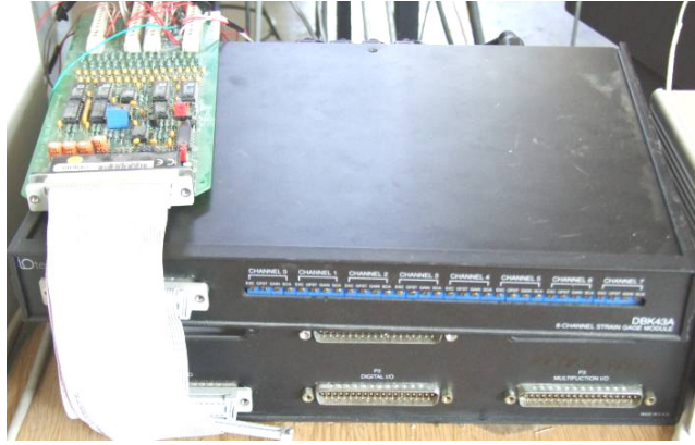
Figure 5.33 DBK80 Analog Multiplexor, DBK43 and DBK43A strain-gage cards
