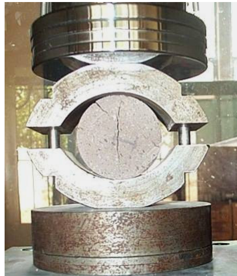
Figure 5. 5 Brazilian test specimen after test
