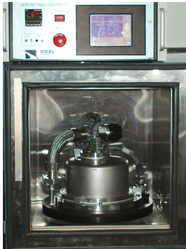
Figure 4.37: Photograph of Ideal Aerosmith 1280 single-axis rate table used for scale factor and linearity measurements of MEMS gyroscopes.
