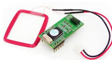
Figure 2.8 RFID module and its receiving wire, which can connect directly to the Arduino via a serial protocol.
